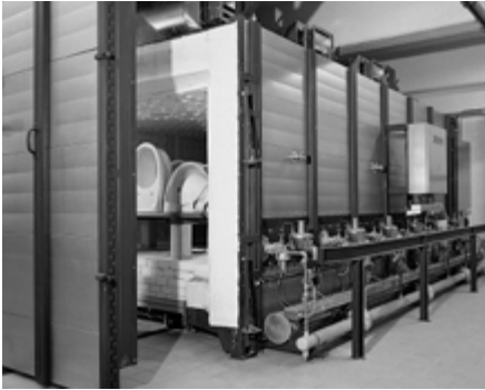
Intermittent shuttle kiln in the ceramics industry
